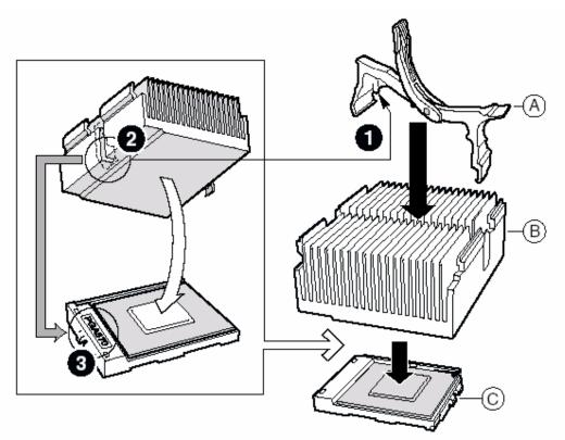
Figure 18: Installing the Heatsink
